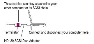
**WARNING** Always disconnect your Macintosh PowerBook from the adapter cable when you are not using it as a hard disk. Your PowerBook will not work correctly if the adapter cable remains attached.
